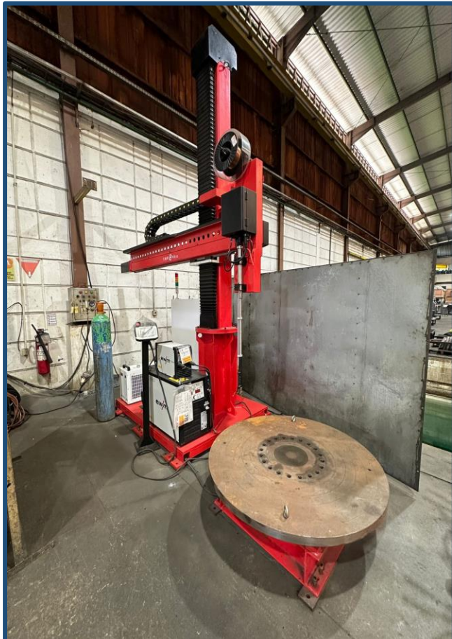
Automatic Welding Machine (GTAW)
